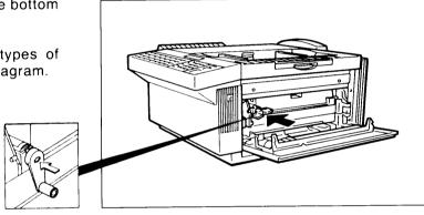
Turn the handle clockwise to remove the seal <u>until you see the yellow band on the</u> <u>seal</u>. Then, remove the handle. Turn until you see the yellow band.
